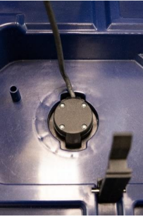
Fig. 59: Guide the monitor cable into the upper shell and carefully pull it taut.
