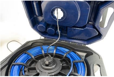
Fig. 60: Wrong: Camera cable not pulled tight
