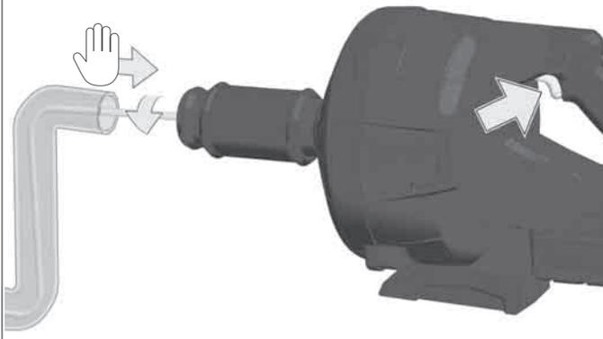
Switch on - cable rotates.
