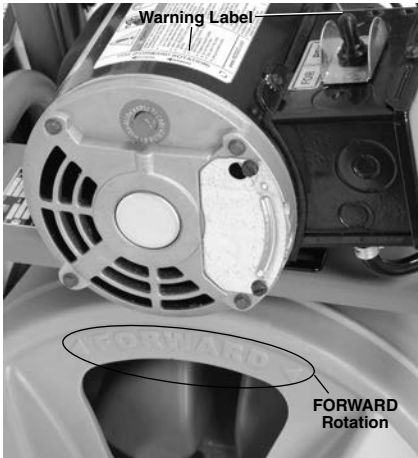
Figure 8 – Proper Drum Rotation (FOR Switch Position)
