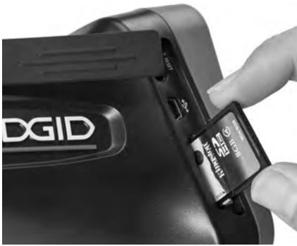
Figure 9 – Inserting the SD Card
