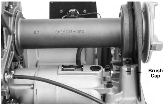
Figure 34 – Removing Motor Cover/Changing Brushes
