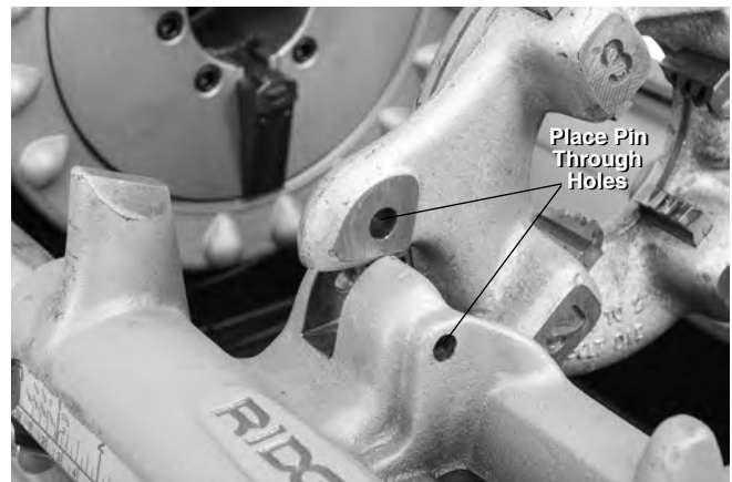
Figure 26 – Retaining LH Die Head in Place
