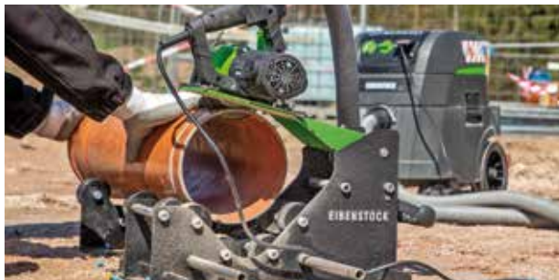
Cutting and chamfering in one step
