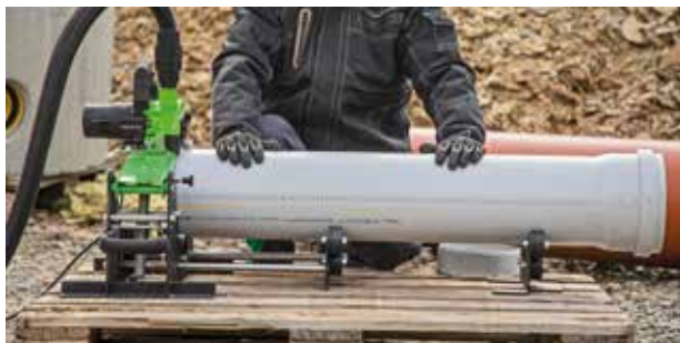
Align the tube horizontally and vertically exactly to the saw blade
