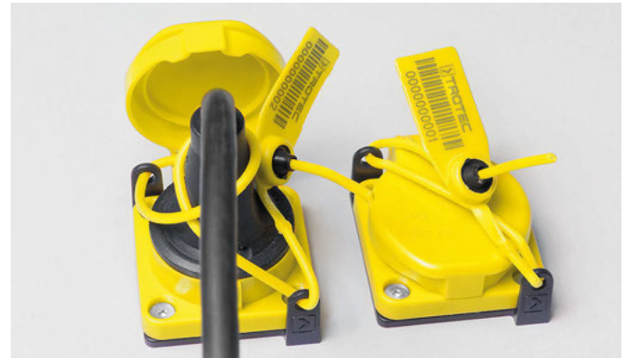
The PlugSafe base plates are designed for built-in sockets with flange mounting. Two opposing, diagonally arranged angle brackets permit the safe application of the socket in accordance with the regulations e.g. by using a consecutively numbered seal. PlugSafe can be used for protection both with an inserted power consumer or when the socket's cover is shut.
