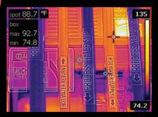
FLIR's patented MSX image enhancement embosses visual details onto full-resolution thermal images in real-time, providing perspective to the scene and allowing you to read text and labels.
