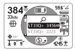
Once a connection is made, the transmitter automatically powers on. When connected, the Bluetooth icon \$ is visible on both the transmitter's and the receiver's screens. On the transmitter, a chain link image confirms that the two units are connected.
