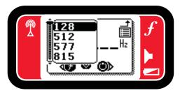
4. Press the Left and Right Arrow keys to move between each digit placeholder and the Up and Down Arrow keys ♠♥ to increase and decrease the values. The ST-33Q+ adjusts the output frequency as each digit is entered. This auto-adjustment allows the tuning of the target frequency for maximum signal at the receiver. Press the Select key ⊚ to save and activate the frequency.
