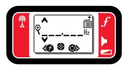
3. Move all the way to the left of the screen to access a drop-down list stored frequencies. Press the Up and Down Arrow keys 🔊 to move through the list. When highlighted, press the Select key 🕲 to input the frequency.
