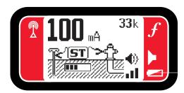
If the display screen shows "Lo," the circuit is open or the unit is unable to draw adequate current for locating. Check your connections and improve the circuit to accurately locate.
