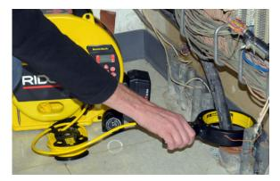
Press the Power key . The ST-33Q+ automatically switches to Inductive Clamp Mode, disables the cable leads, and displays the word "Clamp" on the screen.
