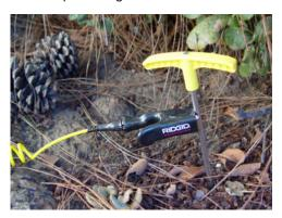
Instead of using the provided grounding stake, the lead clip can be attached to other objects such as a shovel blade or a metal rod sunk into the earth. Using larger grounding objects may improve grounding by increasing the surface area in contact with the earth.
