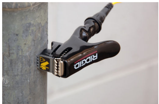
Figure 7 – Connecting the ST-305 using the magnet
