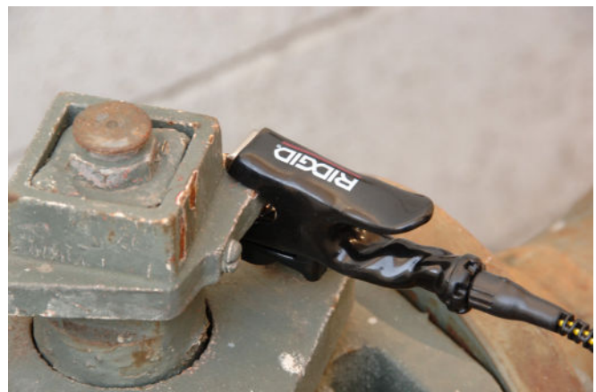
Figure 6 – Connecting the ST-305 using the clip
