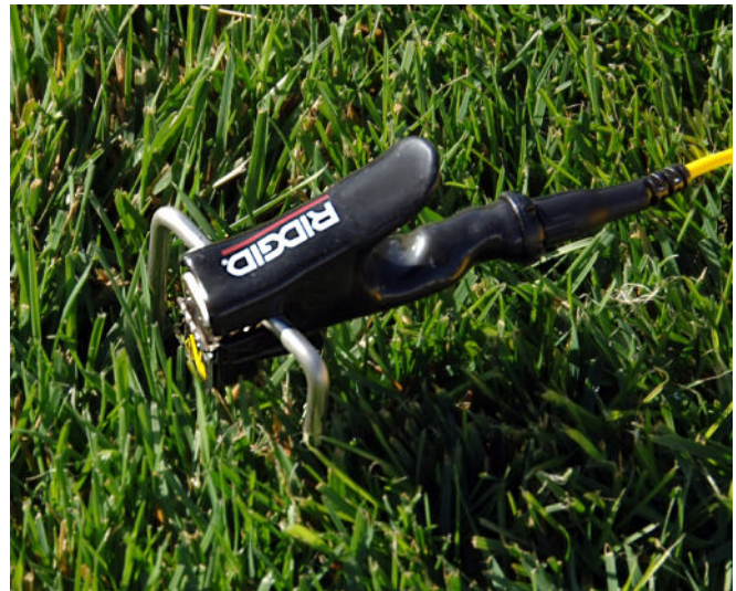
Figure 5 – Connecting the ST-305 Ground Stake
