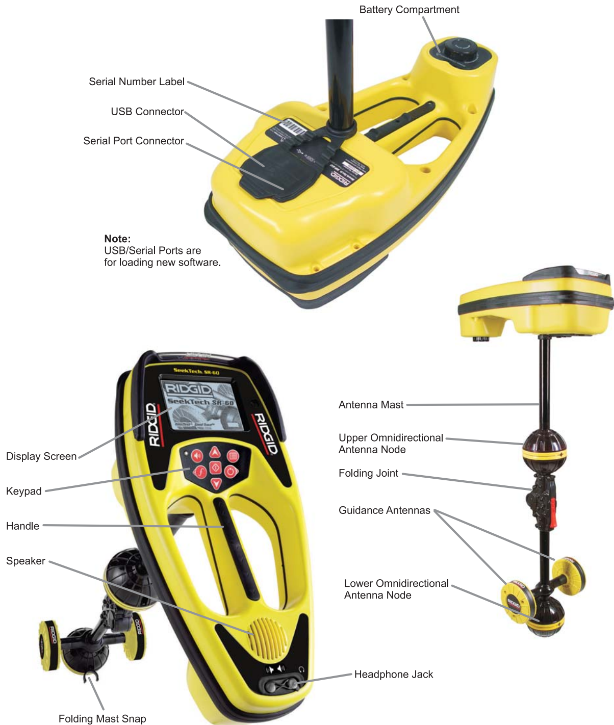
Figure 1: SR-60 Components
