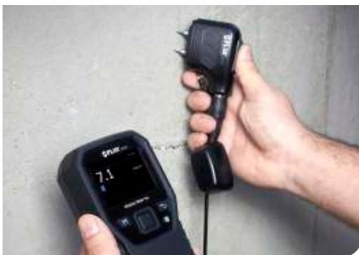
External pin probe for resistive moisture readings
