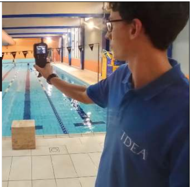
The FLIR MR277 combines the advantages of thermal imaging and FLIR's patented Multi-Spectral Dynamic Imaging (MSX) with advanced environmental sensors to help professionals quickly locate, clearly identify, and easily document moisture problems.
