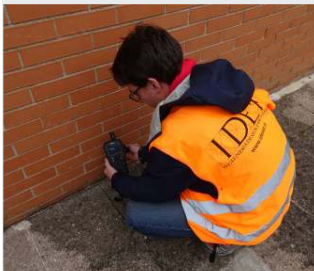
Building professionals can use the FLIR MR277 to prevent problems during the construction phase, for example, to see whether a wall has been dried well enough.
